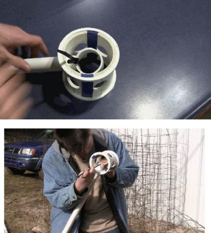
Repeat to attach all 10 Blue Hubs to 10 Blue Struts, and lay the Struts in a stack.
